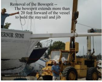
Spars (masts, booms and gaffs, the structures that hold the rigging and sails) are sanded, inspected and repaired.
