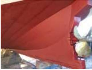
With a new stern post, new prop, four planks partially replaced, caulked and bottom painted, shaft log repaired and drive shaft realigned, she is surely renewed. Thanks to Bill Holland, Teresa Holland Bellais and the staff at Holland Boatyard for their beautiful work.
